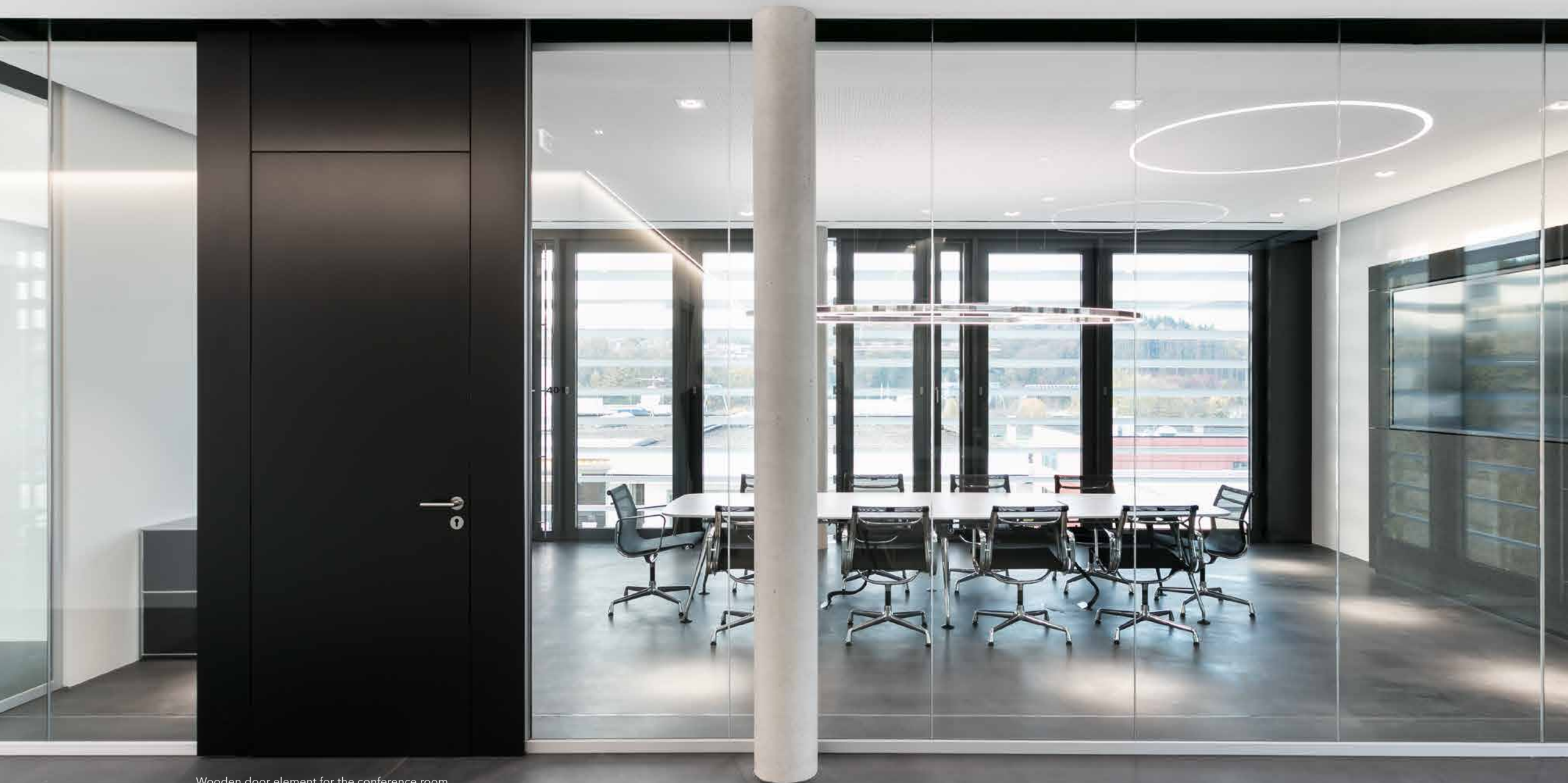
Wooden door element for the conference room with concealed hinges and sound insulation up to 42dB.
